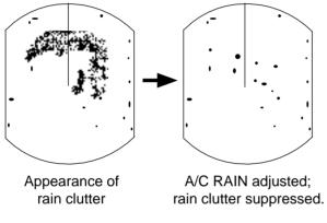
Figure 2-6 Effect of A/C RAIN
